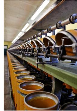
Twisting machine where we inclose individual fibers even more and upgrade the yarn
